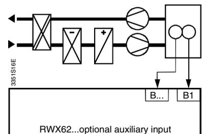
The resulting undercooling of the supply air/room temperature is corrected by the room temperature sequence controller via increased (re)heating.
