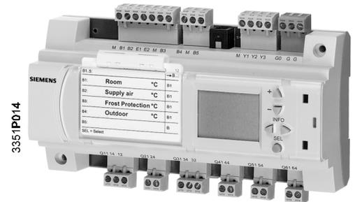
**Fully autonomous electronic universal controller with up to three configurable controllers as sequence controllers with P, PI, PID response or as digital controllers with P-response. Universal inputs for analog or binary signals. Separate outputs for analog or binary signals. AC 24 V operating voltage. Direct entry and setting of all data on the controller; no extra tools required.**
