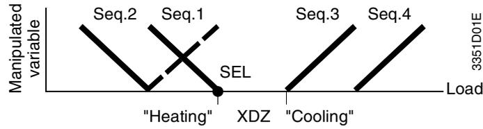
**Operating action** The "Heating" setpoint [SEL] is allocated to the interdependent sequences 1 and 2. Their output signal acts in reverse to the load (input variable), e.g. heating.
