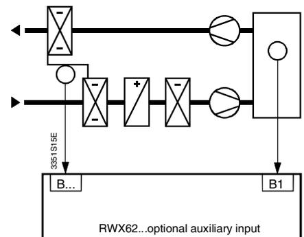
Other typical applications (e.g.): Maintenance of the water inlet temperature in a corrosion-prone heating boiler.
