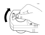
Releasing the lever manually
